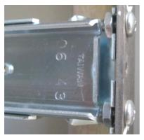
6) Pull out INTERMEDIATE SECTIONS until hits retainer. .
