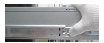
9) Push down TAB on both sides to allow chassis installation.
