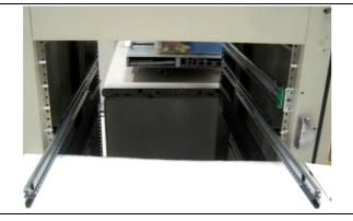
7) Slide in CHASSIS into INTERMEDIATE SECTIONS.
