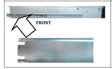
3) Install CHASSIS SECTION BRACKET to both chassis sides with 10-32" screws; slots to the rear side.
