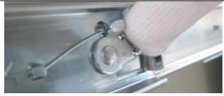
8) Push down lock to allow INTERMEDIATE SECTION rail into FLANGE MOUNT STATIONARY SECTION.
