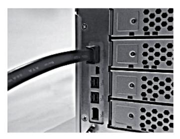
5. Power on the unit via the switch in the rear of the unit.
