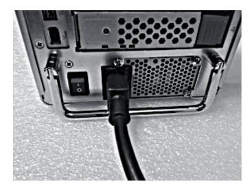
4. Connect one of the data cables from the host to the unit. (USB, Firewire 400, Firewire 800, or eSATA)
