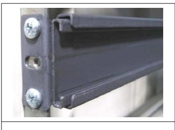
Install Flange mount stationary section, intermediate section must be inserted before end bracket is attached. If cabinet front area is not threaded, use bar nut inside cabinet to hold screws.
