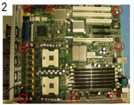
Mounting the motherboard onto the chassis:
