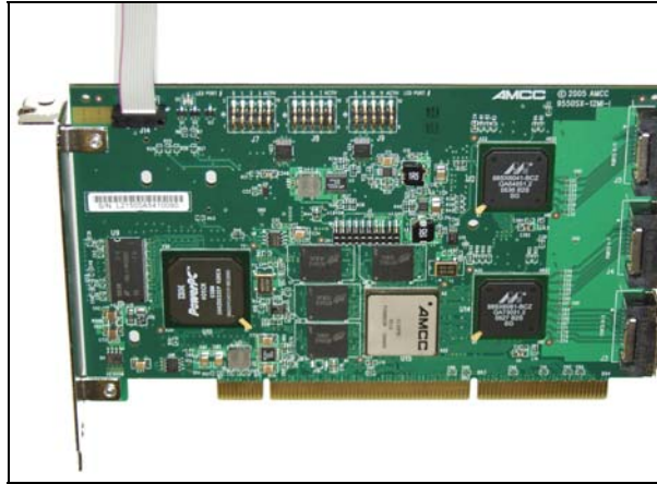
Figure 7 - I2C cable plugged into controller card
