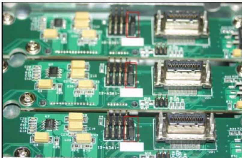
For BP 12-6426-01AR, install also Shunt Jumper on J12
