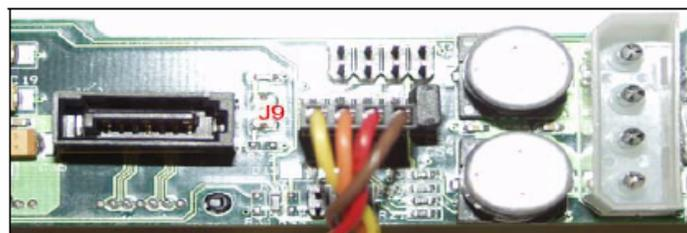
Figure 7 – Cable Installation on backplane
