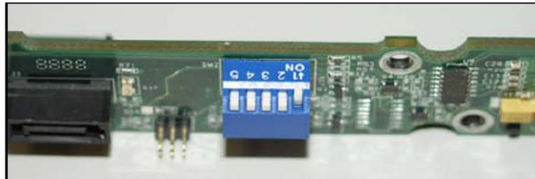
Figure 1 – Turn pin 1 to “ON” position
