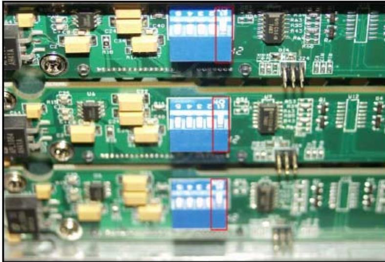
2. Install Shunt-Jumper on Pin 9-10 of J9 (5X2 Header on the Middle of the BP) for all BP.
