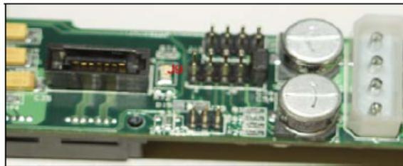
Figure 6 – Installing shunt.
