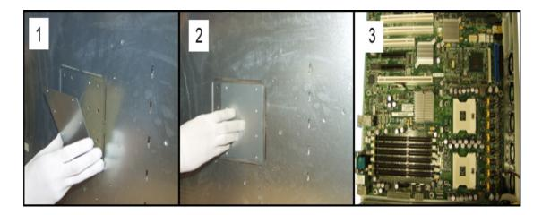
Mounting an Intel® Xeon<sup>™</sup> server board:
