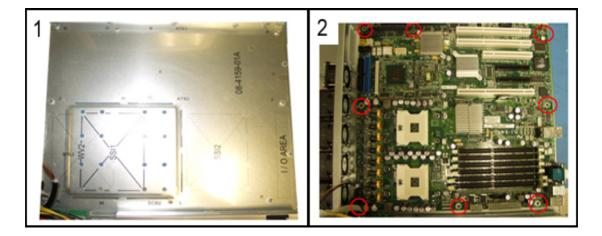
Mounting the motherboard onto the chassis:
