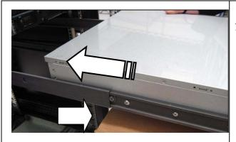
10)Carefully insert CHASSIS SECTION into INTERMEDIATE SECTIONS.
