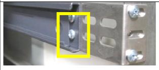
7) Install CHASSIS MOUNTING BRACKET to the rear cabinet section. Screws holding FLANGE MOUNT STATIONARY and CHASSIS MOUNTING BRACKET can be adjust as required. .
