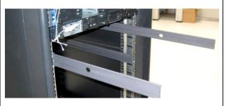
8) Slide out INTERMEDIATE SECTIONS to the lock button.
