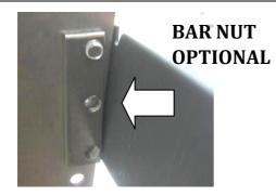
6) NUT BAR is installing when cabinet is not threaded to hold screws.
