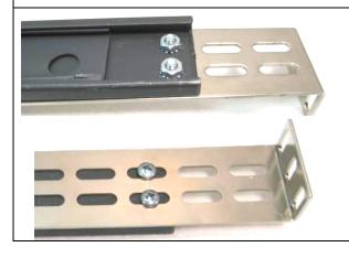
4) Install 06-0330-01A CHASSIS MOUNTING BRACKET to FLANGE MOUNT STATIONARY SECTION.
