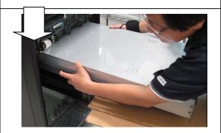
13)Push second lock button to insert complete enclosure into cabinet.
