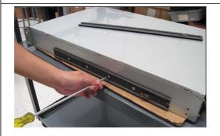
3) Remove and install CHASSIS SECTION with 10-32 round head screws. Lock release to the rear side.
