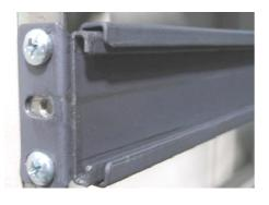
5) INTERMEDIATE SECTION must be inserted into the STATIONARY SECTION before the end bracket is attached. Install bracket to <u>the front</u> cabinet section with 10-32 screws.
