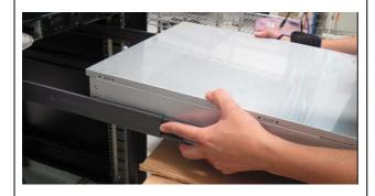
11)Carefully slide bracket pressing lock button to allow CHASSIS SECTION insertion.
