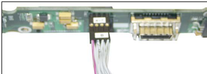
Figure 3 – Activity LED Cable plugged into backplane
